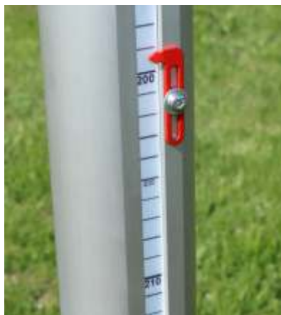
analogue height scale printed on toothed belt with calibrated height arrow
